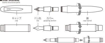
※尾栓にキャップを固定可能です(ネジとめ) The cap can be screwed on to the tail plug of the pen for safe keeping
